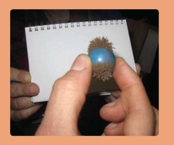
Figure 13: The poles correspond to the area attracting more filings, as this is the area with the highest density of lines of force.
