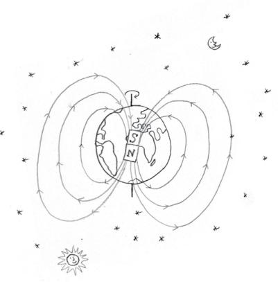
Figure 14: Earth's magnetic field. Interestingly, the magnetic south pole points towards the north.
