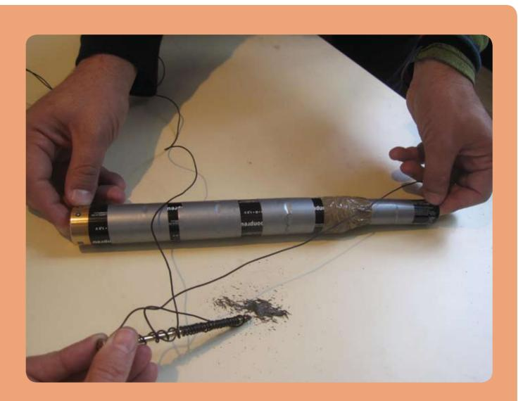
Figure 3: Several batteries connected to an electrical wire to show the movement of the iron chips when current flows.
